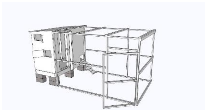
Sample chicken coop design from the Just Food City Chicken Guide. The enclosed area is the coop, and the open area, walled with hardware cloth or wire mesh, is the run. Image courtesy of Just Food.
