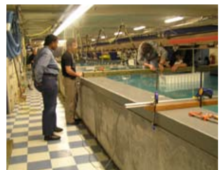
Mounting model onto brace (above) Vertical wall model set up for wave reflection test (below)
